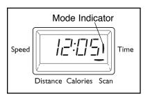
show that the scan mode is selected, and a flashing mode indicator will show which mode is currently displayed. Note: If a different mode is selected, you can select the scan mode again by repeatedly pressing the mode button.
